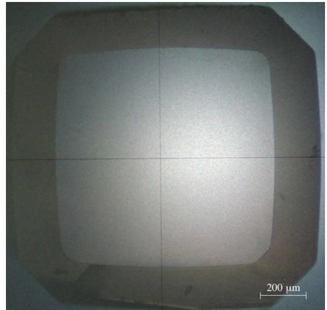
Fig. 1. Cross section of D_h = 1.0 mm square channel.
